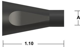
The PL-700 plug housing is designed to accept Amphenol Alden's one piece, Press & Seal PVC Backshell. This unique backshell simply snaps into place providing an IP-67 rated seal to the plug housing and cable exit without hardware resulting in a clean overmolded look. For optimum sealing we suggest selecting a wire exit i.d. that is at least .005" smaller than your nominal cable diameter .
